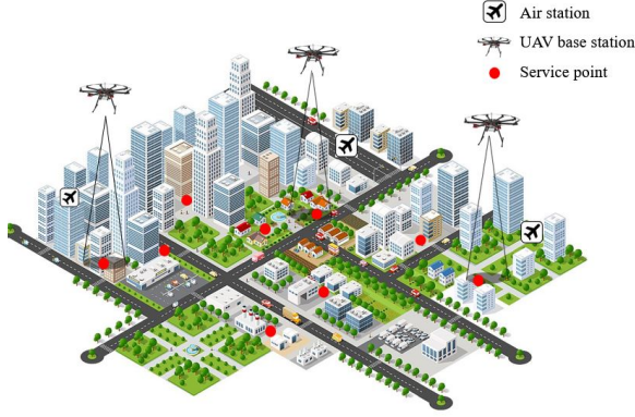
Fig. 1. Multi-UAV assisted wireless network in a post-disaster area.
