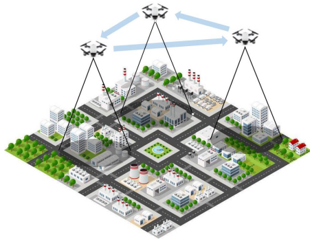
Fig. 1. UAV-assisted emergency communication, where the hovering UAV is utilized as a wireless BS covering a certain area.
